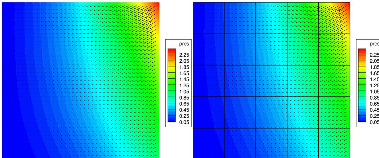
Figure 3: Pressure error (left) and magnitude of velocity error (right) for the multi-scale solution with a single linear mortar per interface in Example 1.
