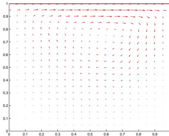
Figure 4: Velocity streamlines for  $Re = 100$ .
