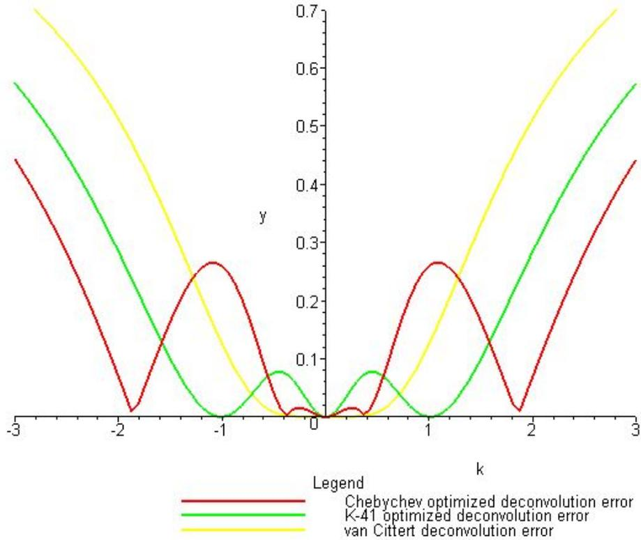
Figure 2: Deconvolution Error (N=2)
